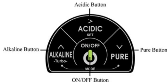
Simple controls make using the Revelation a breeze! There are four levels of alkaline water, four levels of acid water, and a pure water button.
